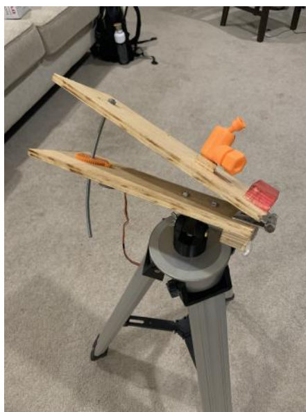
The current version 3 design of the tracker with the curved screw and 3d printed eq-wedge.
