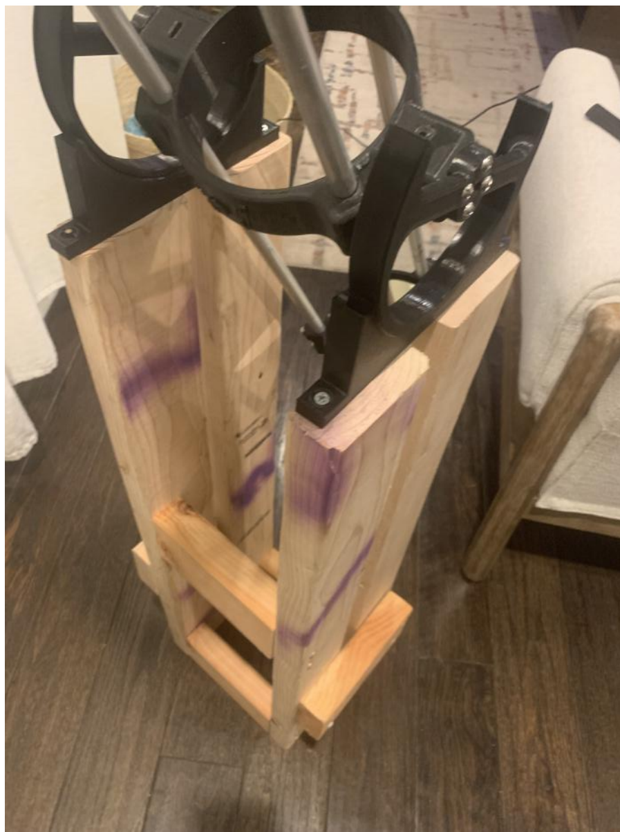
Original 2x4 base design with 3D-printed Dobsonian bearings.
