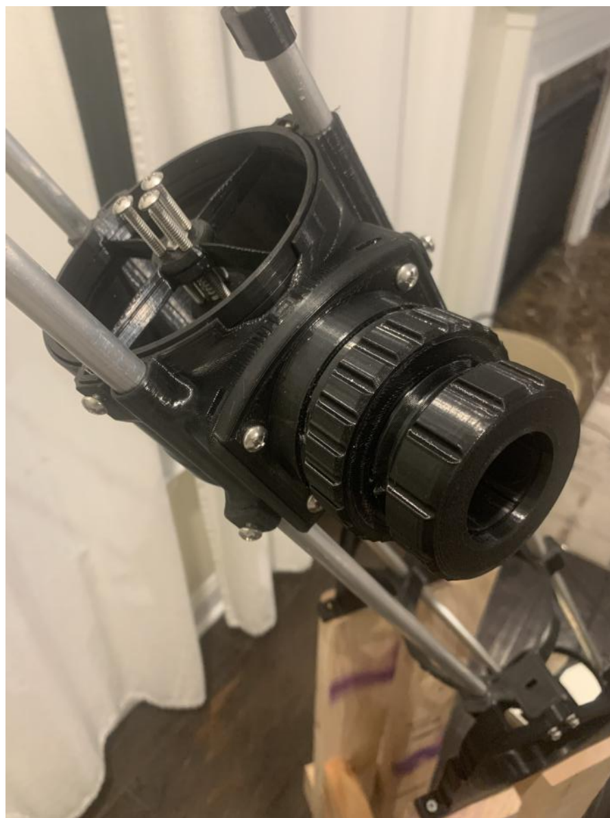
The 3D-printed non-rotating 1.25" focuser with the Hubble-style 4-vane spider and three-screw adjustment mechanism.
