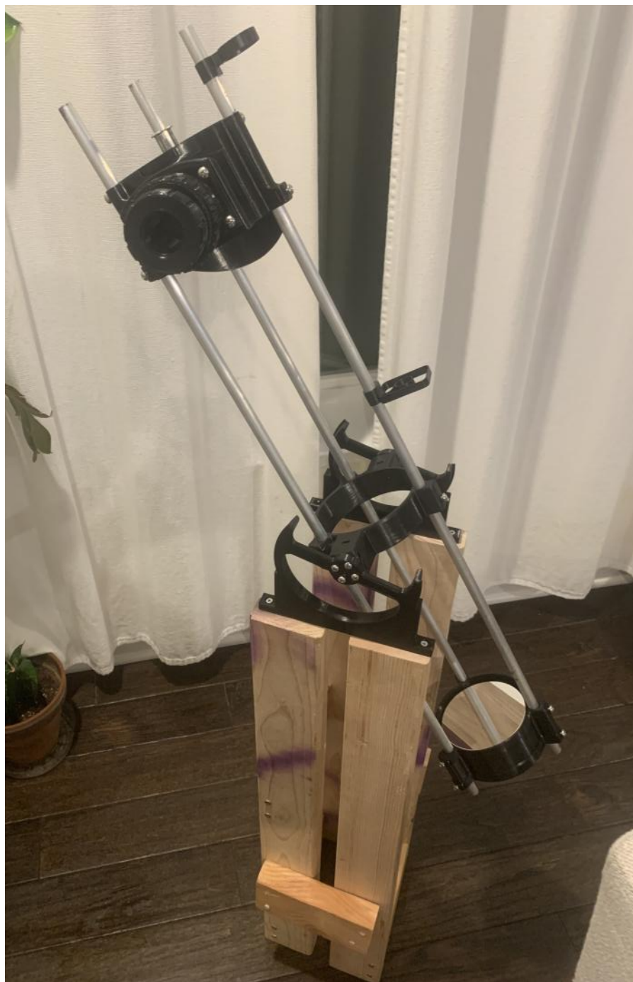
The complete Hadley 114 telescope, with the three major parts, UTA, MTA, and LTA, as well as the 2x4 base.
