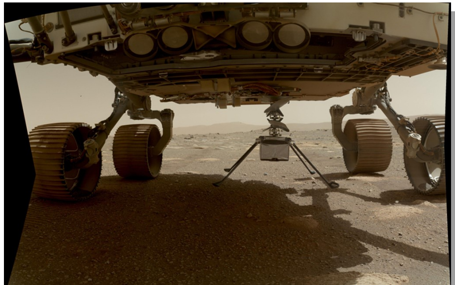
The Mars Ingenuity Helicopter, all four landing legs down, was captured here on sol 39 (March 30) slung beneath the belly of the Perseverance rover. The near ground level view is a mosaic of images from the WATSON camera on the rover's SHERLOC robotic arm. Near the center of the frame the experimental helicopter is suspended just a few centimeters above the martian surface. Tracks from Perseverance extend beyond the rover's wheels with the rim of Jezero crater visible about 2 kilometers in the distance. Ingenuity has a weight of 1.8 kilograms or 4 pounds on Earth. That corresponds to a weight of 0.68 kilograms or 1.5 pounds on Mars. With rotor blades spanning 1.2 meters it will attempt to make the first powered flight of an aircraft on another planet in the thin martian atmosphere. 1 percent as dense as Earth's, no earlier than April 11. Image Credit: NASA / JPL-Caltech / MSSS
