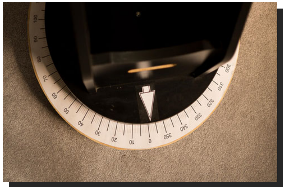
Step 6: Put arrow mark perpendicular to the axis of rotation of the optical tube.
