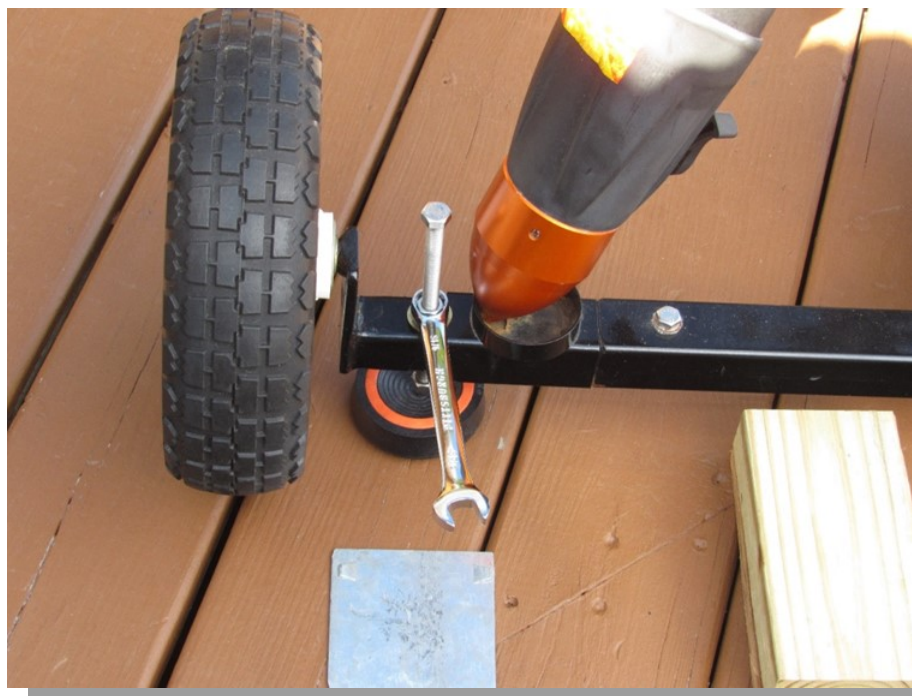
Tightening the nuts with the box-end wrench.
