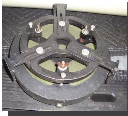
Mirror in its Cell with Adjustment Points
