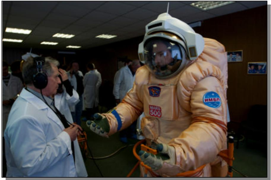
Testing a Martian version of the Orlan spacesuit used in the Mars500 experiment. The suit has been modified for use in Earth gravity. Photo Credit: S. Corvaja, 2010 (ESA).
