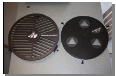
Spike-a Bahtinov mask next to the author's conventional three triangle Hartmann mask.
