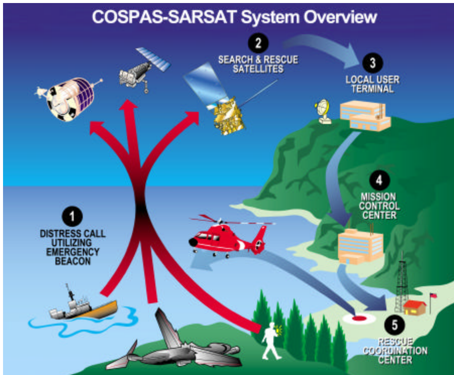
NOAA's polar-orbiting and geostationary satellites, along with Russia's Cospas spacecraft, are part of the sophisticated, international Search and Rescue Satellite-Aided Tracking System.
