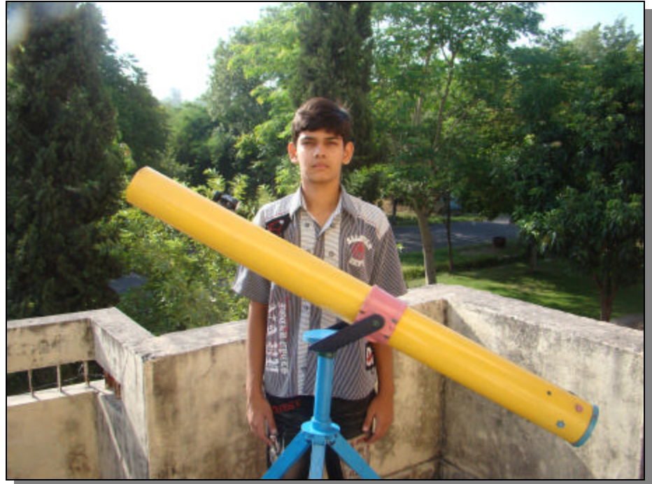
Ekam Noor Singh and one of the two telescopes he has built, a 100 mm diameter Newtonian reflector.
