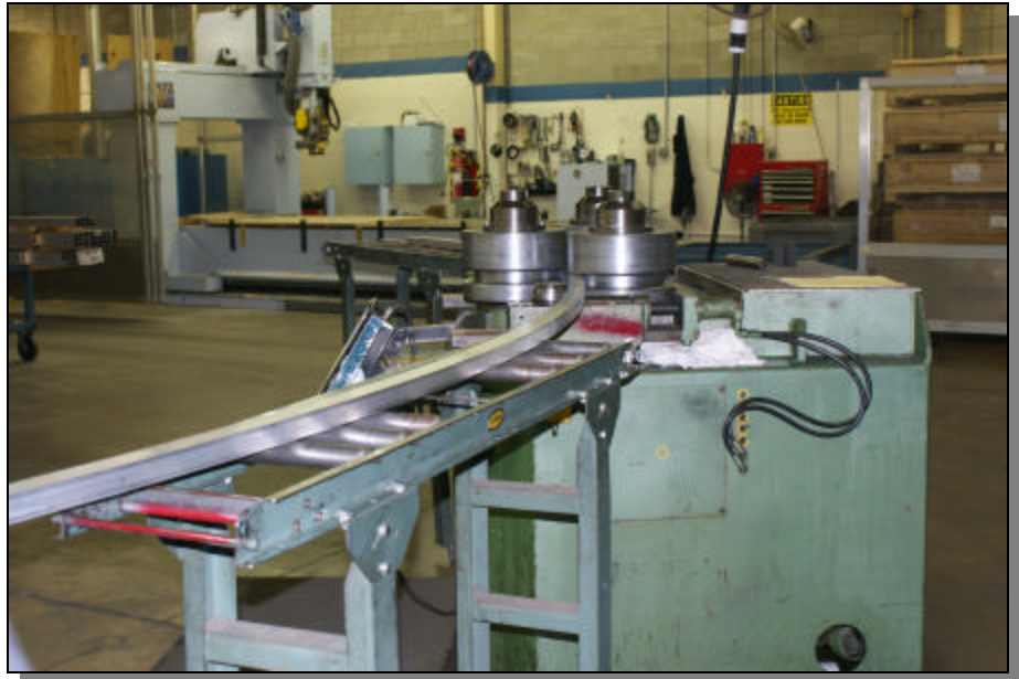
The manufacturing facility at Spitz, Inc. is a "cold facility", e.g. no heat is used in the fabrication of the dome components. All parts are shaped using "brute force".
