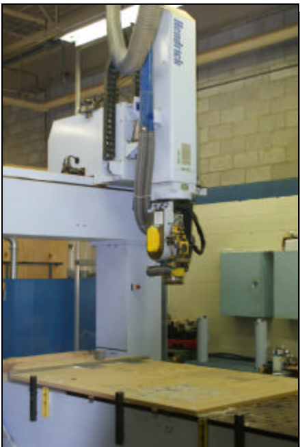
The cutting machine used to fabricate the panels for each unique dome project.
