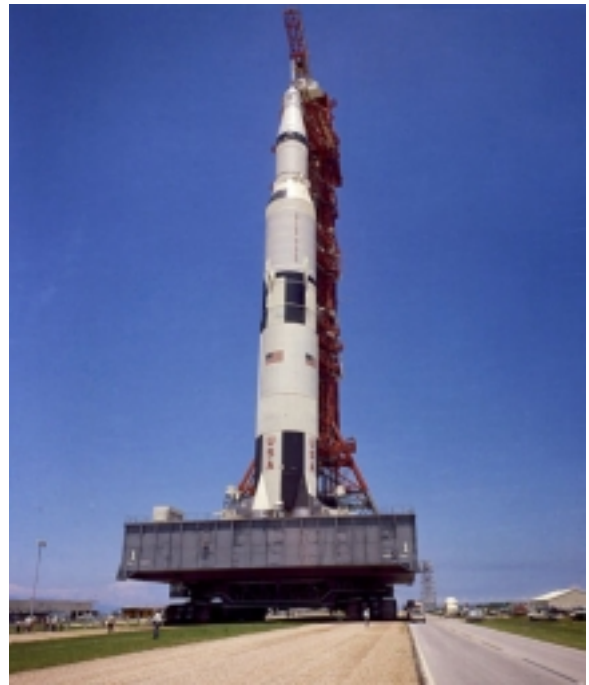
The Saturn V and Mobile Launch Platform are carried to the launch pad on the Crawler Transporter. Notice the tiny humans below the platform.
