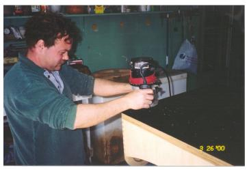
Here we see Steve Lurcott, again on March 26. The Formica sheet has been cemented to the bottom of the rocker box, and then rolling pins were used to smooth it out and press out air bubbles. Now that the cement has set firmly, Steve is using a router to trim the edges of the Formica. Ed says that "Steve is the carpenter in the family".
