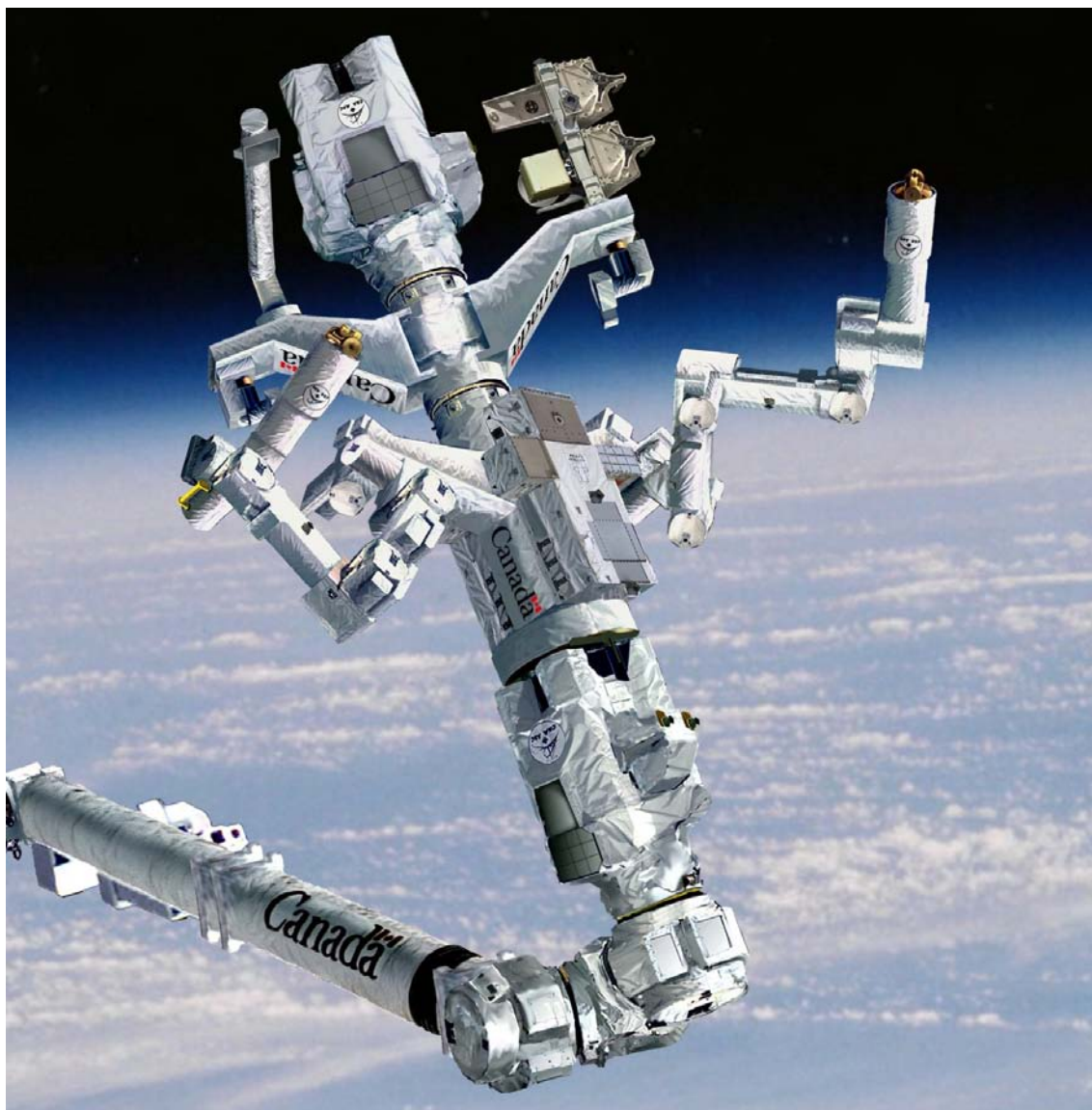
The Special Purpose Dexterous Manipulator can perform delicate human-scale tasks such as removing and replacing small exterior components.
