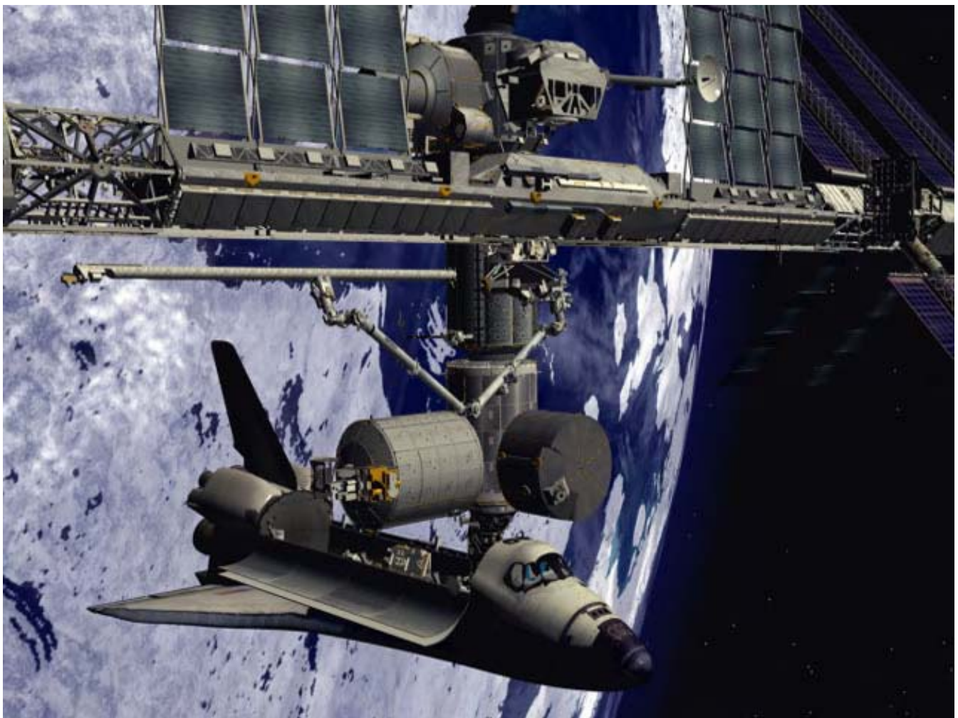
This image illustrates the station's robotic arm grappling the Orbiter Boom Sensor System in preparation for its temporary stowage on the station's S1 truss.
