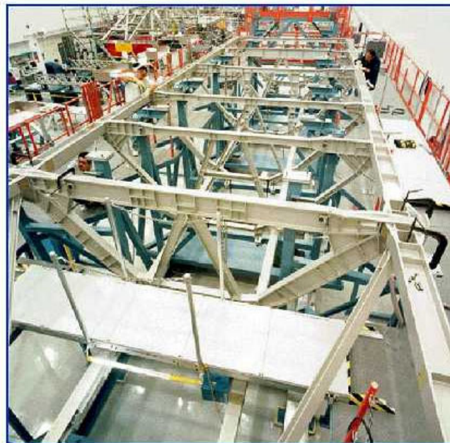
Frame of S1 structural test article at Boeing facility in Huntington Beach, Calif., circa 1998
