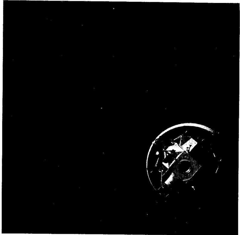
FIGURE 1-4. — The LM is shown in place on the SIVB stage shortly after separation of the CSM and the SIVB stage. (NASA photograph AS12-50-7329)
