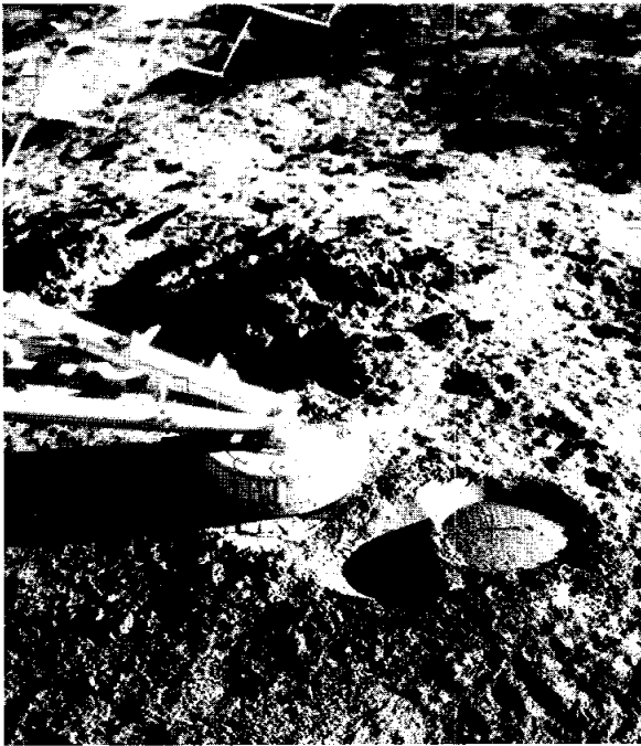
FIGURE 10-69. — Surveyor 3 footpad area, showing footpad prints formed during touchdown hop. Note fresh appearance of the footpad prints and the waffle pattern caused by the footpad honeycomb. (AS12-48-7110)
