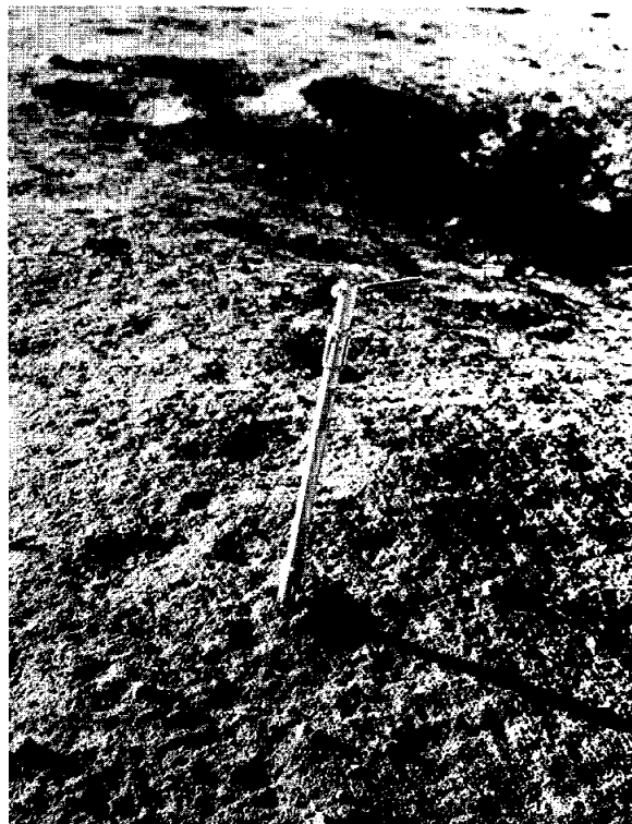
FIGURE 10-67. — Double-core tube at the completion of driving. No disturbance of the surrounding surface is evident as a result of driving the core tube. (AS12-49-7288)
