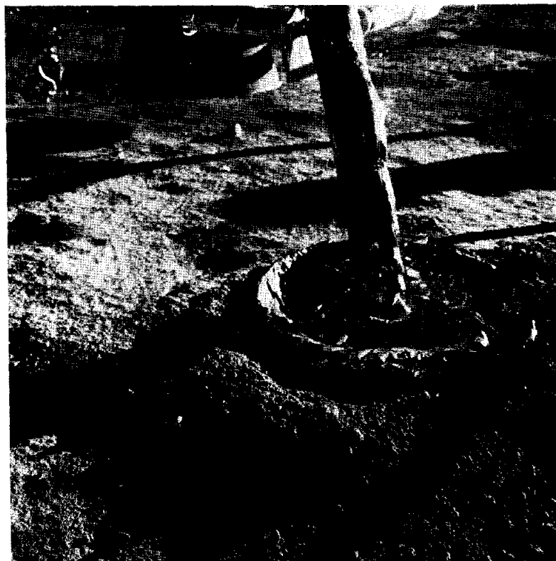
FIGURE 10-53. — Penetration of -Y footpad. (AS12-47-6901)
